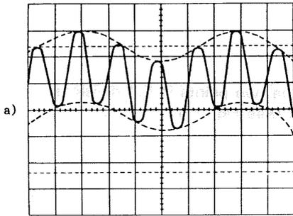
a) Signal containing undesired component
