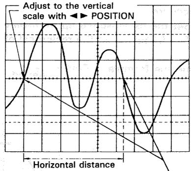
Fig. 13 Adjust to the vertical scale with  $\blacktriangleleft \blacktriangleright$  POSITION
